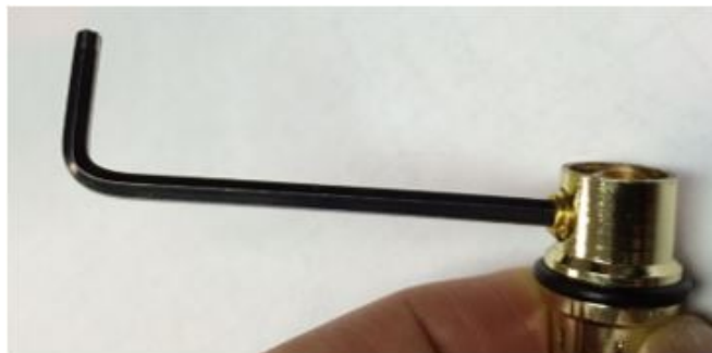
Figure 5: Adjusting the Fuse Set Screw
